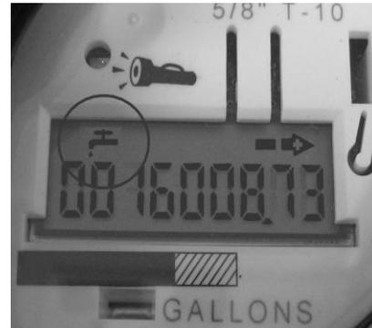
shining a flashlight on the meter face plate. The new meter stores data at 15-minute intervals and allows the meter to identify intermittent or continuous leak
